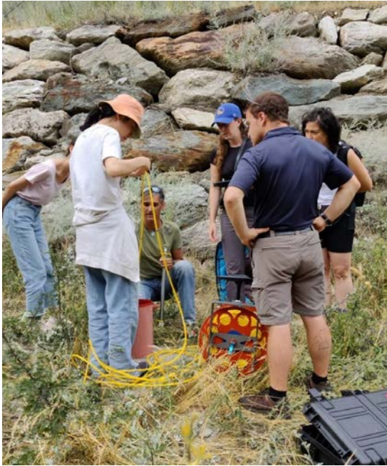
Figure 5. Inclinometric measurements conducted by the students at the Landslide of Baise Pierre during the field trip of Friday 8th
