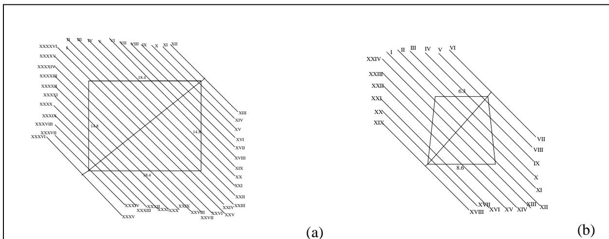
Figure 4: Plans that represent the exact place of the boreholes in relation to a) the building, which includes the tomb and b) the tomb.
