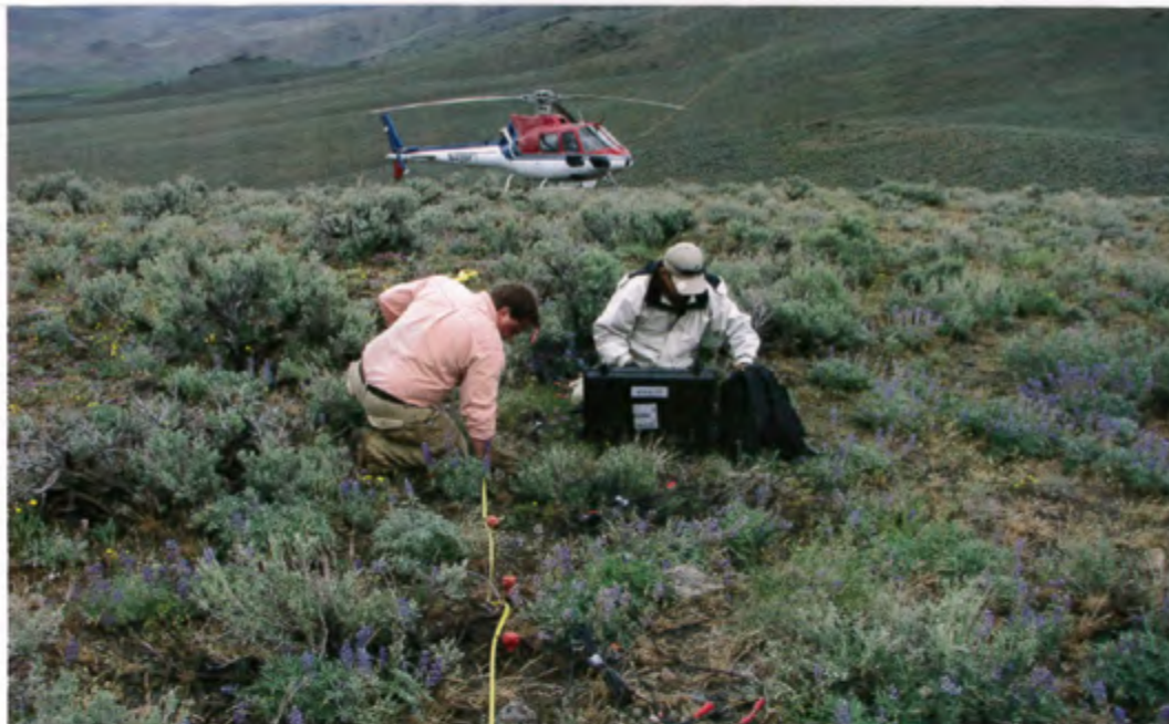
Seismic refraction survey used to forecast rock excavation for design of a pipeline in Humboldt County, NV.
