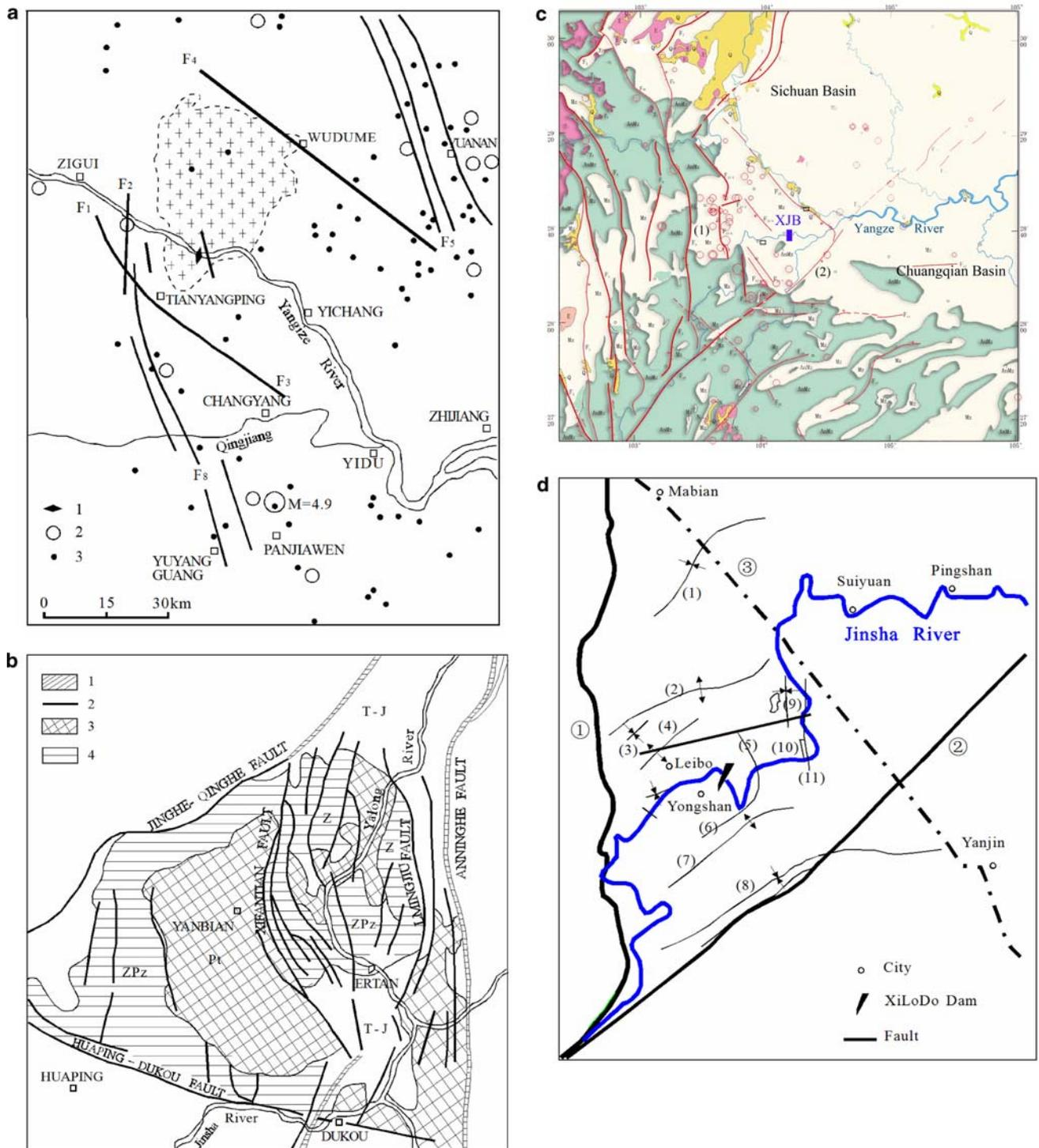
Fig. 8 Seismic geo-hazard level of studied cases: a Three Gorges Project (dam site,  $2 M \geq 4$ ,  $3 M < 4$ ), b Ertan hydropower station (major faults, 2 minor faults, 3 Pre-Cambrian rocks, 4 Palaeozoic rocks), c Xiangjiaba hydropower station, d Xiluodu hydropower station
