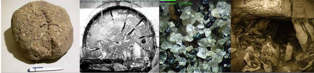
Figure 3. A clay ball from the excavation chamber of a Tunnel Boring Machine (TBM) (left) – note pen for scale. Clay stuck to the cutting wheel of a TBM (middle left). Long straight, convex and concave contacts characteristic of ancient sands (middle right) (P. Verhoef, with permission). Large scale collapse of an abandoned room and pillar calcarenite mine in South-Limburg, the Netherlands (right, from Bekendam, 1998)
