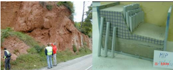
Figure 4. Description of weak rock mass during the Spanish fieldwork (left). Using the centrifuge to examine the performance of innovative methods of dike stabilisation (right).
