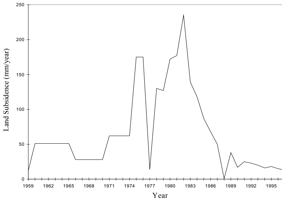
Figure 2. Variation of the annual land subsidence from 1959 to 1997 at BM Bu 435 (a long-term monitoring point in Tanggu, Tianjin)
