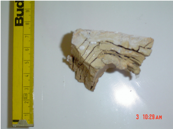
Figure 1. The effect of 5 cycles of immersion of brick in sodium sulphate solution followed by drying in oven
