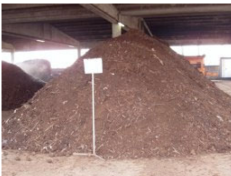
Figure 3. Product obtained by residual sludge bioremediation process
