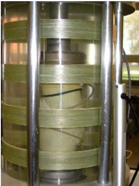
Figure 3. Destroyed sample \phi 50 mm in cell
