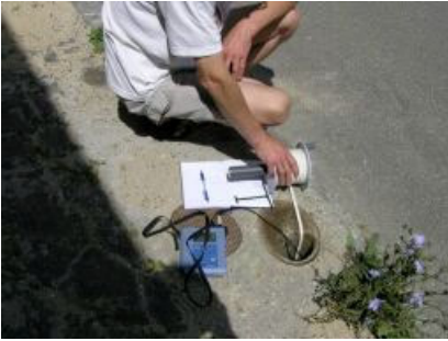
Figure 1. Measuring water level, temperature and pH value of the ground-level observation well in Pécs
