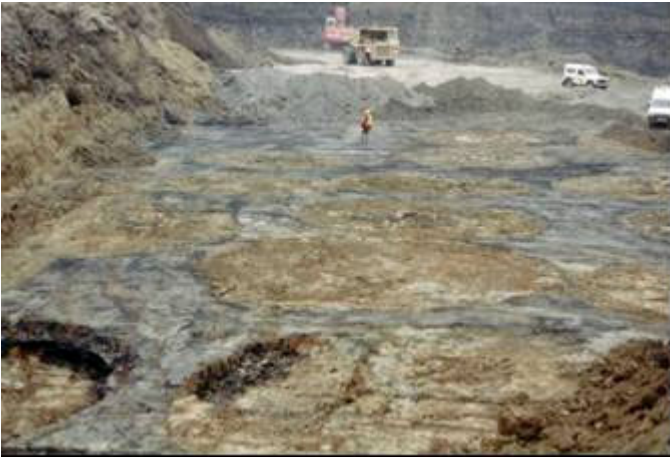
Figure 2. Bell pit workings uncovered during opencast operations at a site near Wakefield. (Photo courtesy of Carl Drury, The Banks Group).
