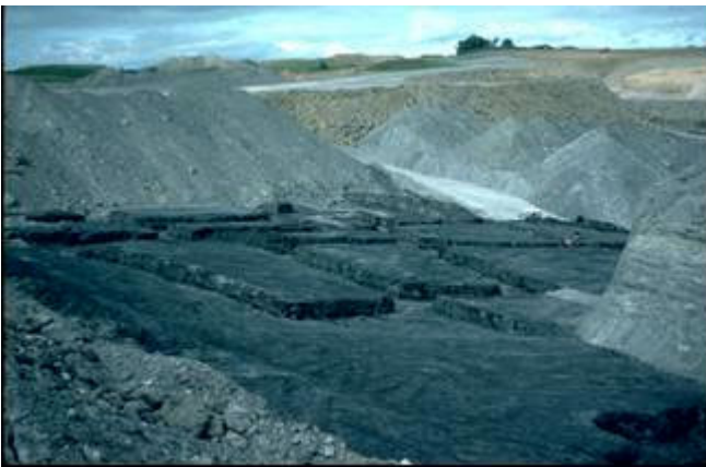
Figure 3. Room and pillar workings uncovered during opencast operations at Buckhead Site, Co Durham
