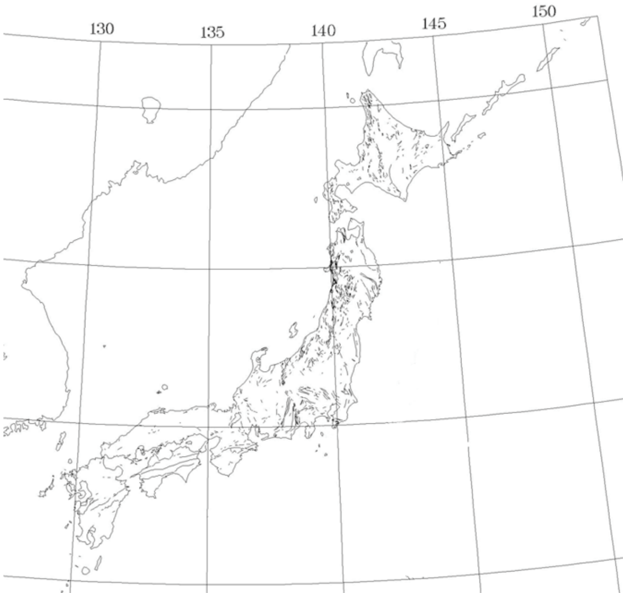
Figure 8. Distribution of on-land faults
