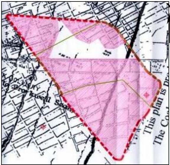
Fig 2. Extent of recorded workings in the Brockwell seam, located approximately 236 mBGL. The site's boundary is shown in red dots, the coal mine workings are shown in red shade. One recorded mine shaft, and room and pillar workings are recorded on the site. (source of original mine plans: The Coal Authority).
