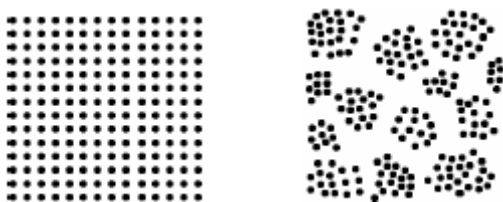
(a) Homogeneous ( D_{corr} = 1.79 ) (b) Clustering ( D_{corr} = 1.54 ) Figure 3. Example for demonstrating the degree of clustering by correlation dimension
